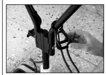
Hang the power cable in the strainreliever Plug the cable into the power
